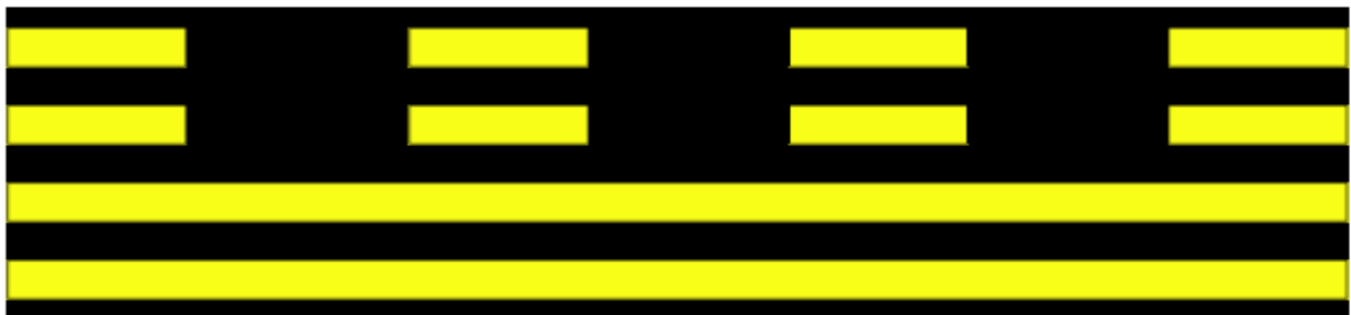
Figure 13.1 Runway Holding Position Marking
